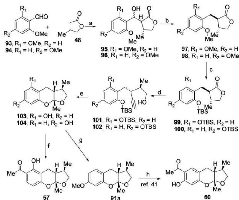
**Scheme 18.** Synthesis of Xyloketal D (**57**) and Xyloketal G (**60**)
